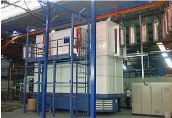
The boilers are being transported respectively the first and second spraying station, where they are clamped to secure proper entering of the application lances.
