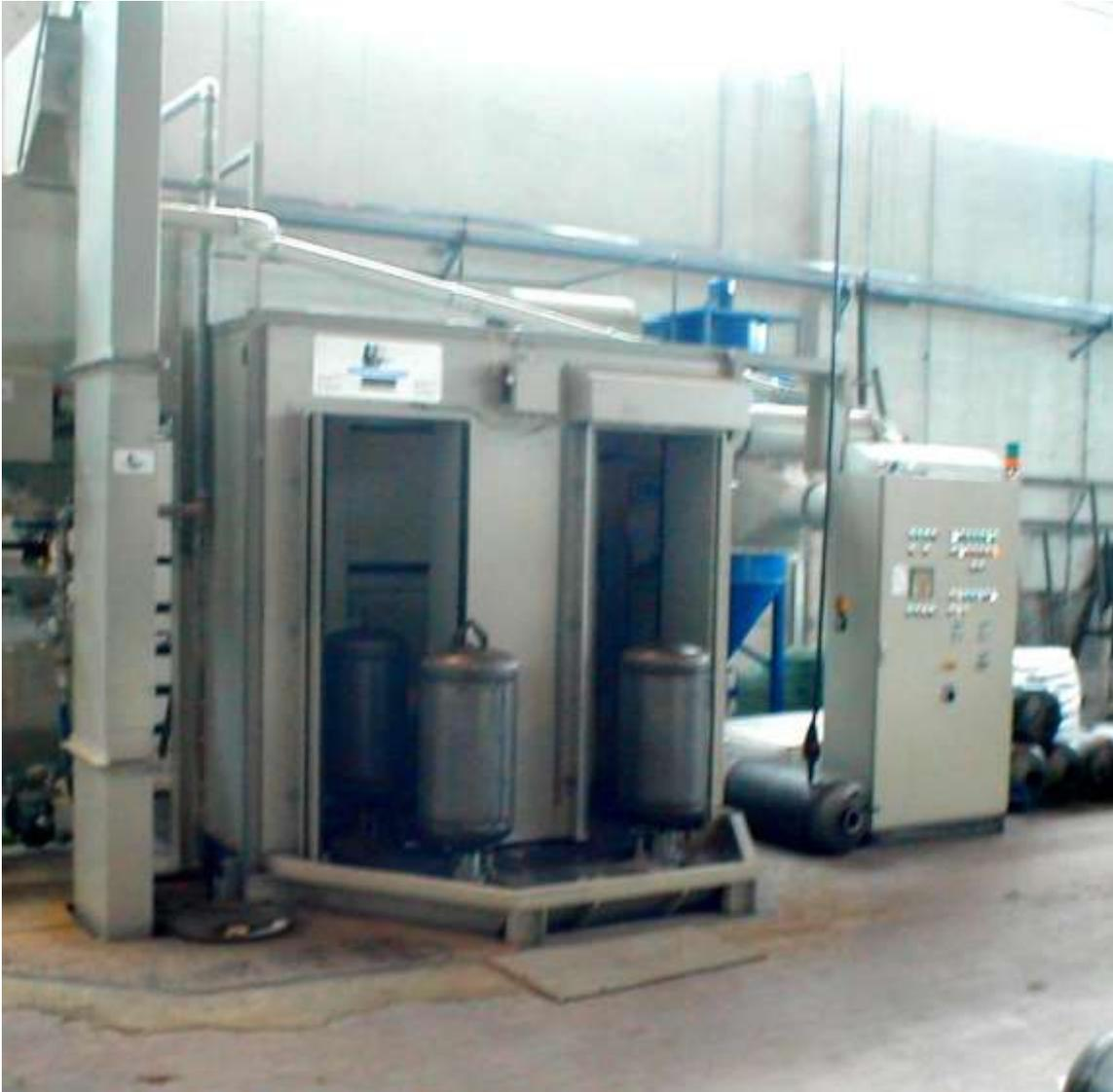
Once the products have been clamped to the table, the operator has to select the appropriate program and push one button to initiate the blasting process, which is done fully automatically in accordance with the data stored in a Siemens S7 PLC.
