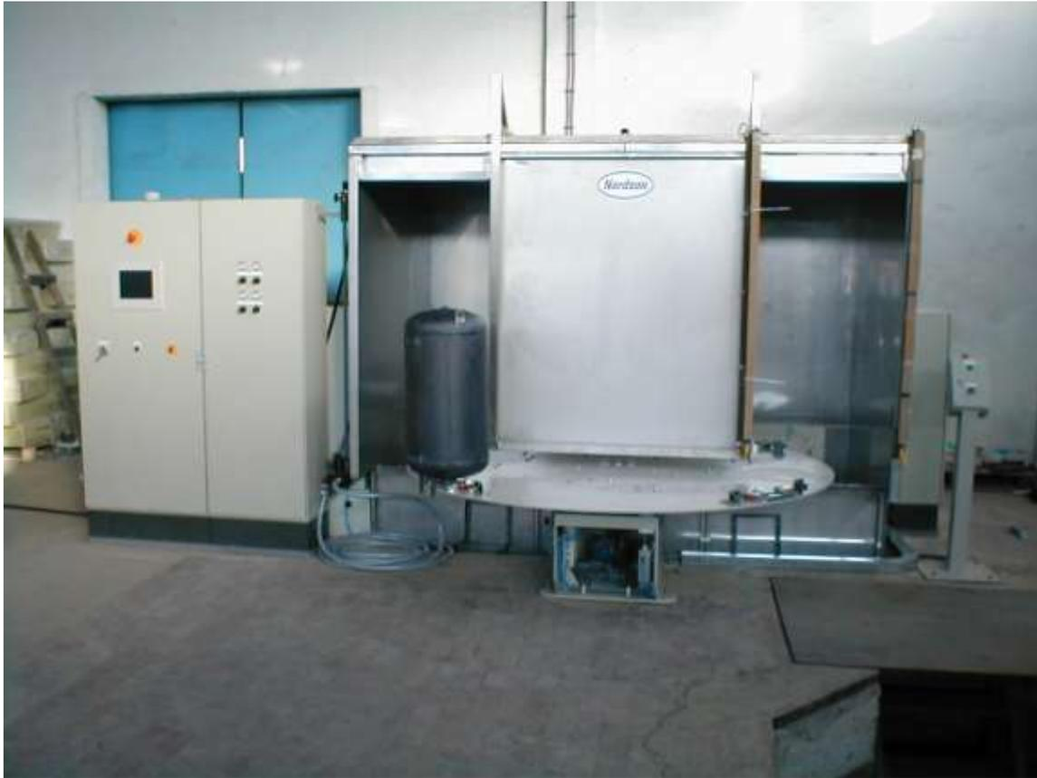
The system, which has two application stations and may be operated by one person, has a typical production of 30 to 40 boilers of 80 liters per hour, depending upon the product complexity & application requirements.
