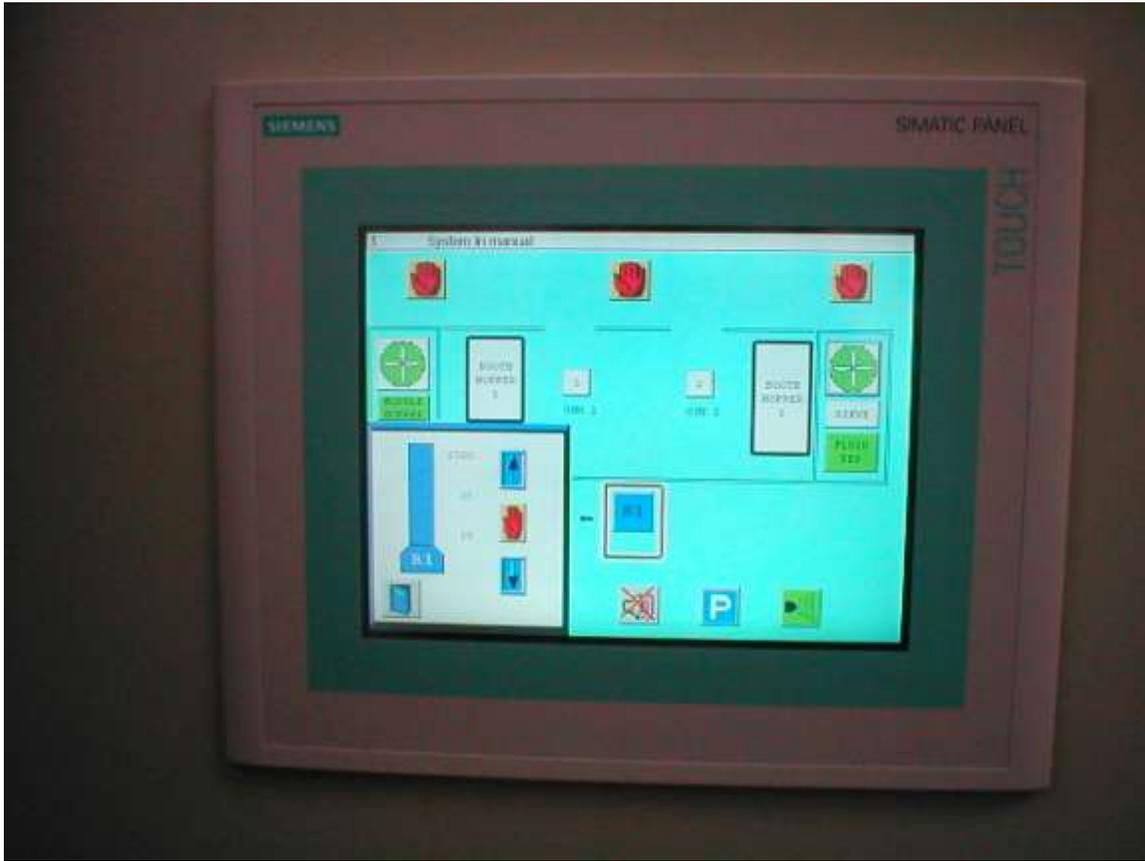
This allows even a relative inexperienced enamellist to produce a good & constant quality once the right process parameters have been entered into the controls system.
